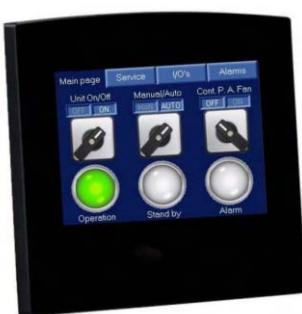
The simple to use PLC main page contains three "buttons" and three indication lights...
