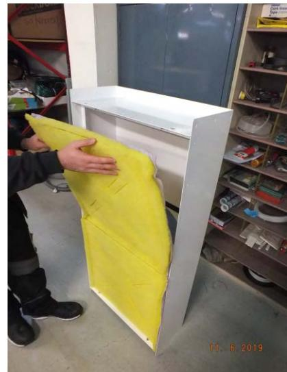
An example of a custom made filter box made for a Coolstore installation of Dehutech Dehumidifier. An additional filter was required to prevent fine particles from forklift operations entering the dehumidifiers.
